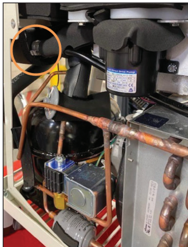
Fig. 8-22 Disconnect two clamps (Step 3- DC pump)
