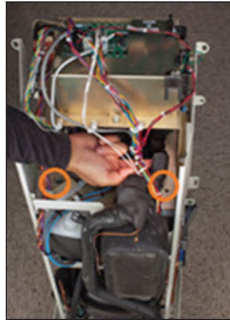
Fig. 8-17 Remove two bolts (Step 2)
