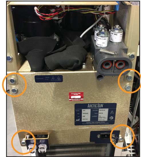
Fig. 8-36 Remove six bolts (Step 3)
