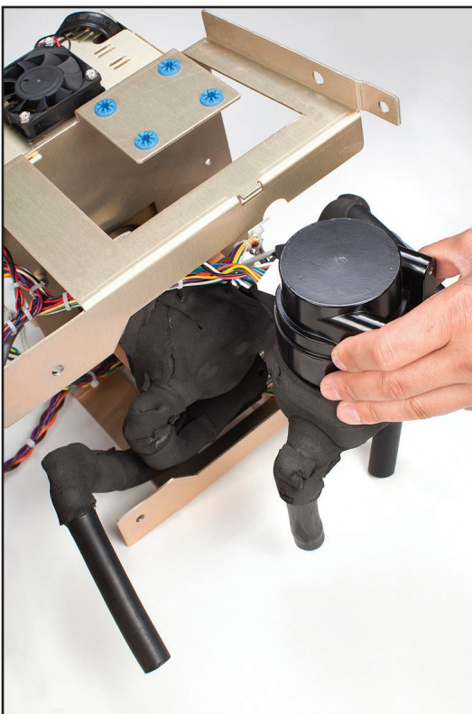
Fig. 8-31 Carefully remove the Mixing Pump (Step 5).
