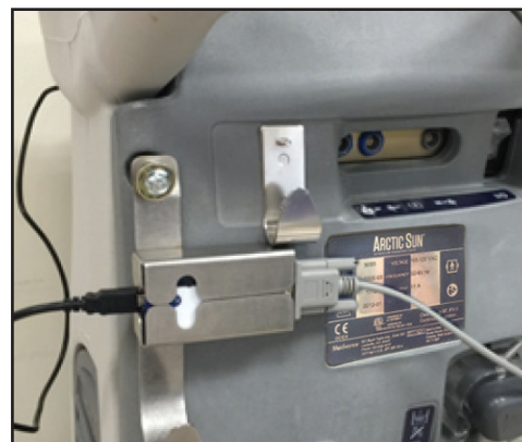
Fig. 8-74 Insert TIM and connect cables (Steps 3-5)
