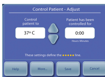
Fig 1-8 Control Patient - Adjust panel (appears after user presses Adjust on Control Patient panel)
