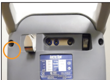
Fig. 8-72 Remove bolt (Step 1)
